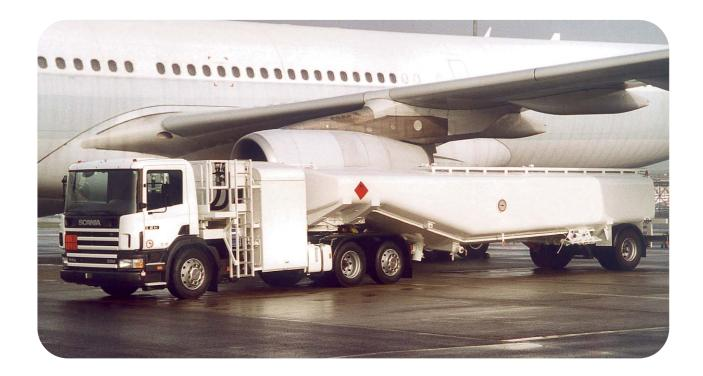
In the past 20 years the Alfons Haar Aircraft Refuelling Unit ARU has proven itself as the very successful concept of modular design for aircraft refuellers. The ARU comprises all required refueller components including pump, filter water separator
